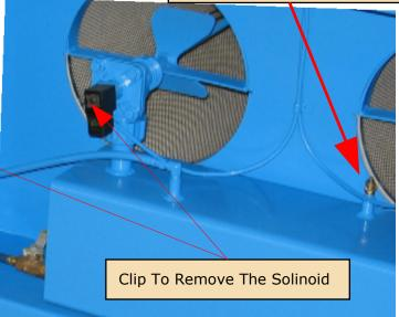
Solinoid to activate the valve 120 Volts
