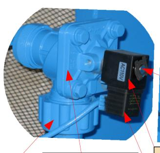
Valve to release air into the filters to clean them
