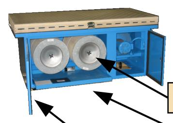
The filters will clean better with machine off, you may shut machine off and before it slows down to a complete stop, pulse the filter and allow the fan to prevent the dust from exiting the filter compartment.
