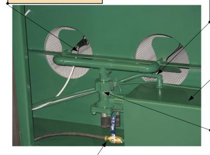
Compressed air inlet into tank 100-140 PSI
