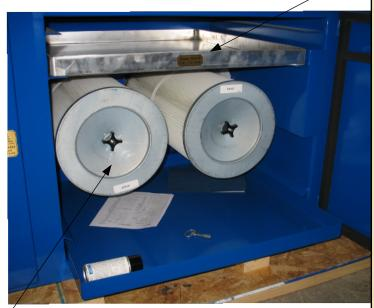
Filters in GRIND tables are SPUNBOND MEDIA 100% polyester. This media has a much higher cloth to air ratio, and cleans better by pulsing than paper or blended media. The efficeincy is 99.95% at .5 Micron.
