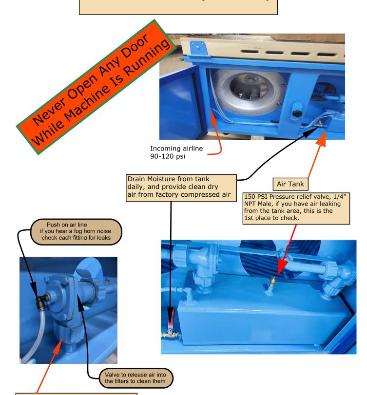
Compression nut that holds valve to the tank. Always apply a small amount of either grease or oil to the threads when reassemling to the tank.
