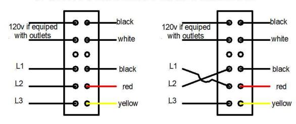
When the fan is going the wrong direction you can loose up to 50% of the suction.
