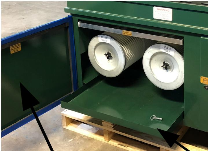
The filters will clean better with machine off, you may shut machine off and before it slows down to a complete stop, pulse the filter and allow the fan to prevent the dust from exiting the filter compartment. Filter replacement number is on the inside of the filter door. Be sure to replace with same type of filter or a filter made of polyester media.
