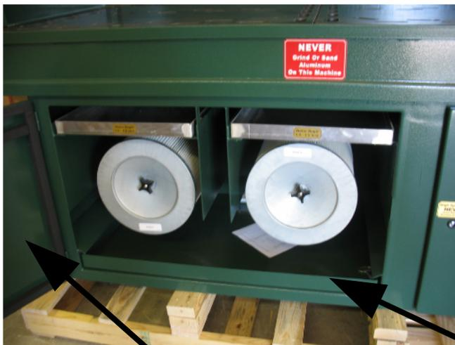
The filters will clean better with machine off, you may shut machine off and before it slows down to a complete stop, pulse the filter and allow the fan to prevent the dust from exiting the filter compartment.
