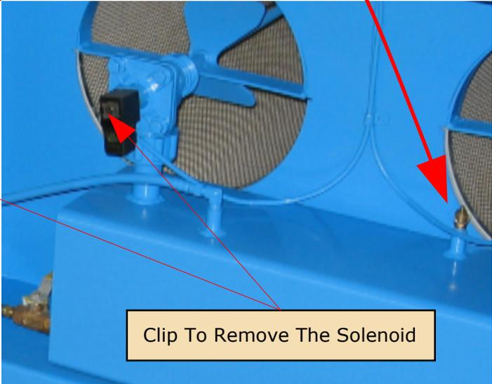
Clip To Remove The Solenoid
