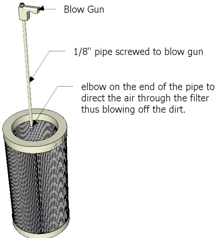
Filter Cleaning is almost the only thing that has to be done to maintain these machines. No lubrication to maintain. The cleaner the filters are kept the better the machine will perform. The dirtier the filters the harder it is to pull air through them.
