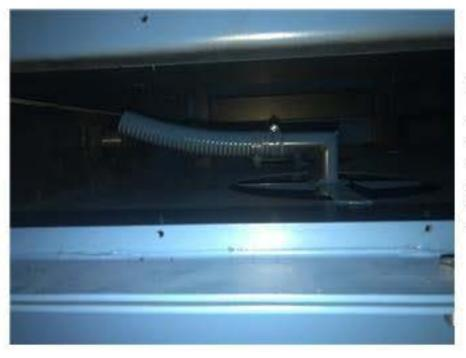
On each end /side there is a small panel held on with the 5/16" hex headed screws that opens to the hoses that leads to the air tank, remove the panel and you will see the hose that fits on the hosebib. placing the hose over the bib and tightening the hose clamp to secure the hose, so the filters can be pulsed cleaned.
