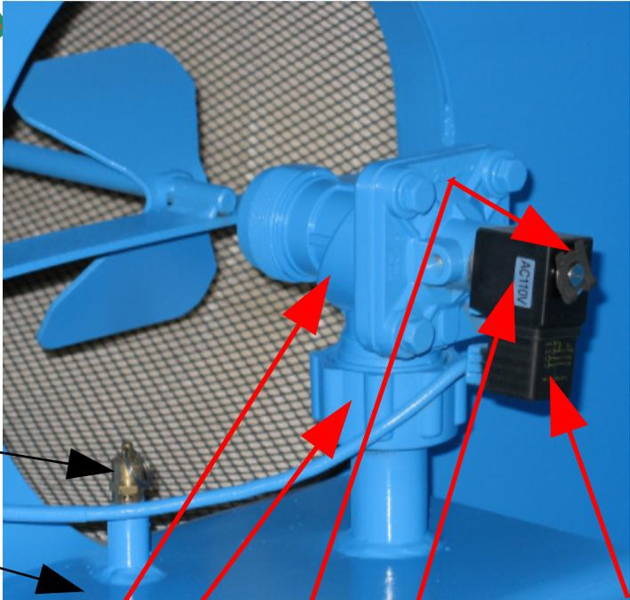
Electrical Plug that screws on the solenoid by one screw
