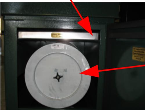
The filter is made from a Spunbond media. The media has been treated with a fire retardant chemical. To help prevent from adding fuel to the fire. This does not mean the filter is fire proof, because the debris on the filter will be the fuel
