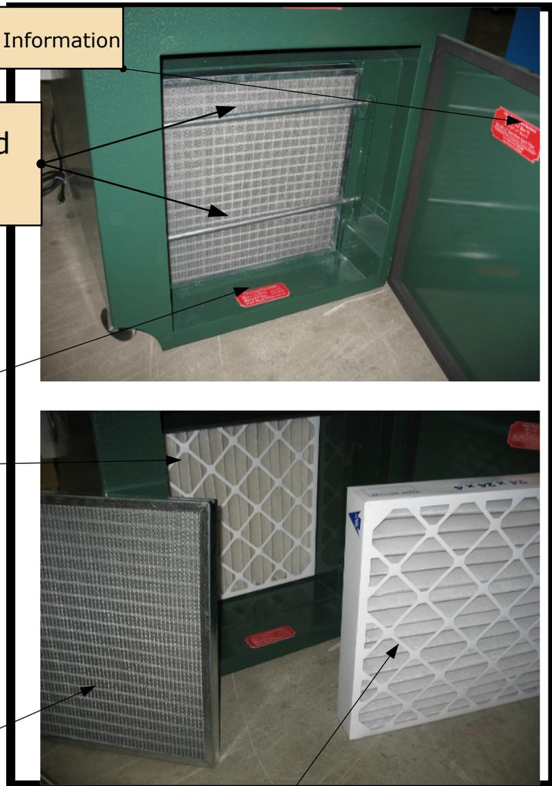
The Merv 8 filter is the MIDDLE filter and it will capture the bulk of the dust particulates. Most of what goes through it will get captured in the back or third filter. The spark filter is designed to HELP PREVENT sparks from getting to the filters behind it. It is not an absolute spark STOPPER.
