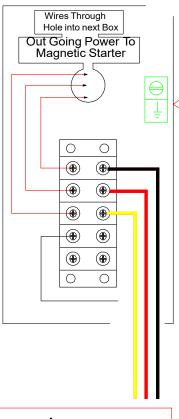
Box on outside of machine for easy wire hook up
