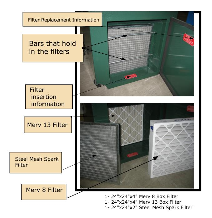
The Merv 8 filter is the MIDDLE filter and it will capture the bulk of the dust particulates. Most of what goes through it will get captured in the back or third filter. The spark filter is designed to HELP PREVENT sparks from getting to the filters behind it. It is not an absolute spark STOPPER.
