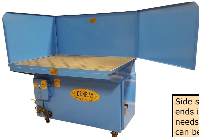
Side shields can be opened on the ends in the case of a long item needs to be processed. The ends can be removed if desired.
