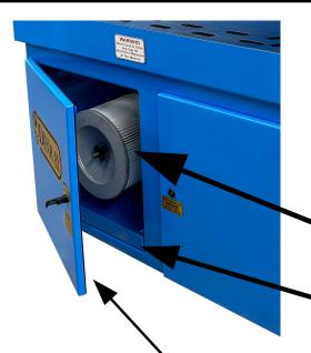
The filters will clean better with machine off, you may shut machine off and before it slows down to a complete stop, pulse the filter and allow the fan to prevent the dust from exiting the filter compartment.
