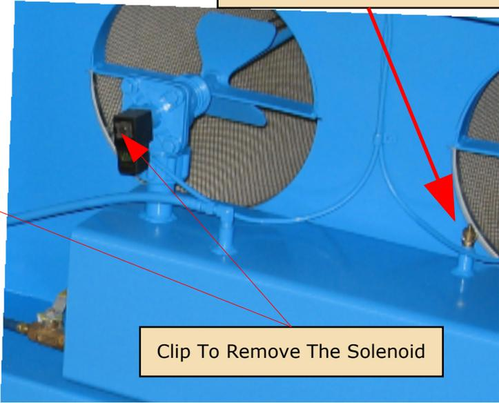
Clip To Remove The Solenoid
