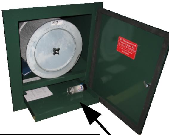
The filters will clean better with machine off, you may shut machine off and before it slows down to a complete stop, pulse the filter and allow the fan to prevent the dust from exiting the filter compartment. Filter replacement number is on the inside of the filter door. Be sure to replace with same type of filter or a filter made of polyester media.
