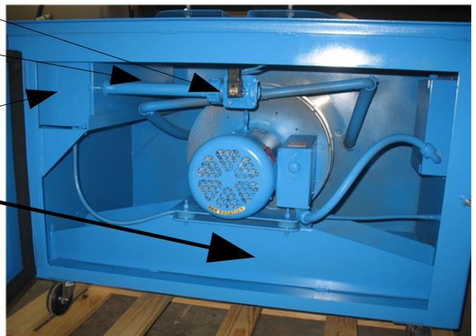
The exhaust air will exit through opening to the floor, if muffler is added the plate on the end will be located here to force the air through the muffler
