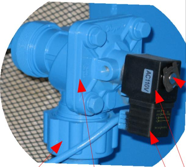
Clip To Remove The Solenoid
