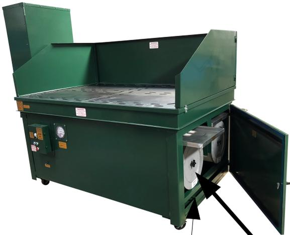
The filters will clean better with machine off, you may shut machine off and before it slows down to a complete stop, pulse the filter and allow the fan to prevent the dust from exiting the filter compartment. Filter replacement number is on the inside of the filter door. Be sure to replace with same type of filter or a filter made of polyester media.
