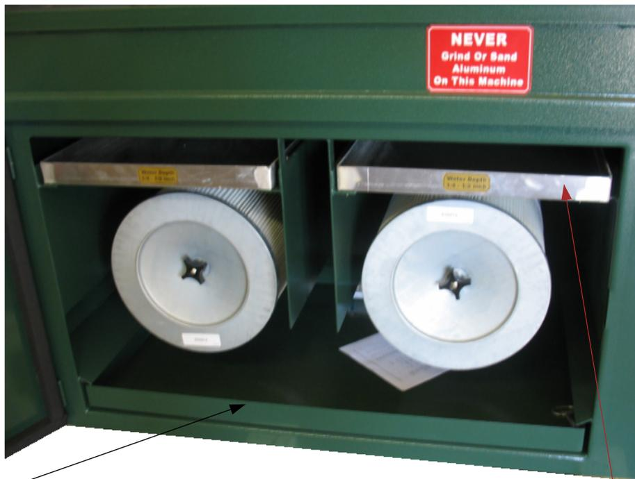
Dust pans will accumulate what is blown off the filters
