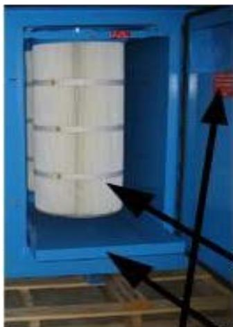
The filters will clean better with machine off, you may shut machine off and before it slows down to a complete stop, pulse the filter and allow the fan to prevent the dust from exiting the filter compartment.
