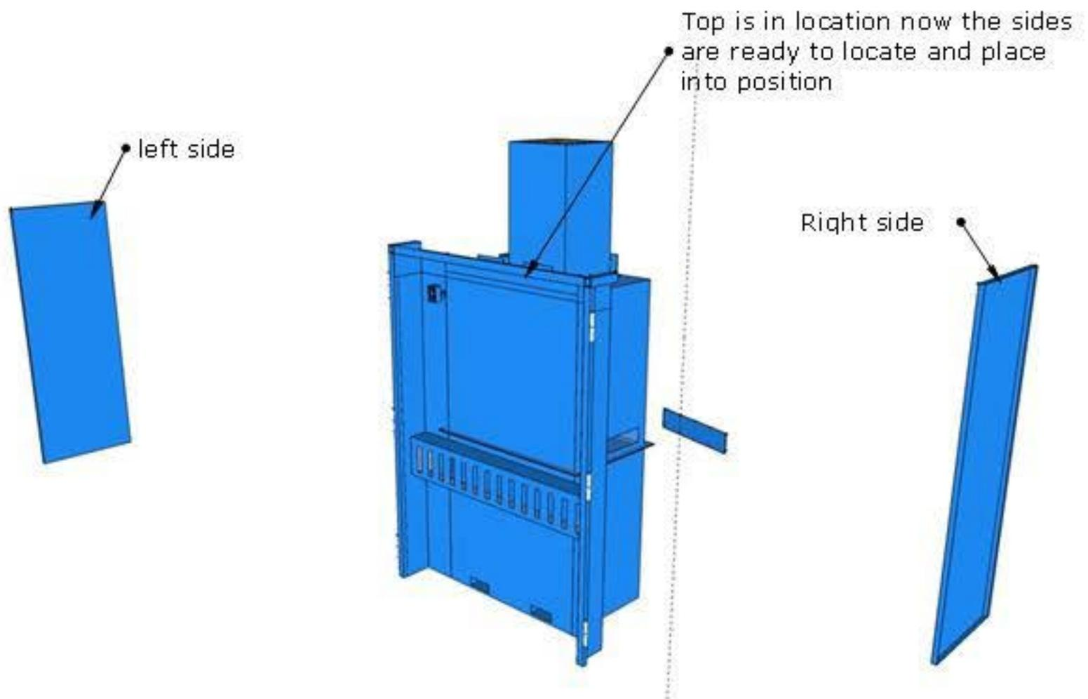
Weld on hinge is what secures the sides, just slide the pin into the hole. Lubrication like WD 40 will help allow the side to slide into hole better.
