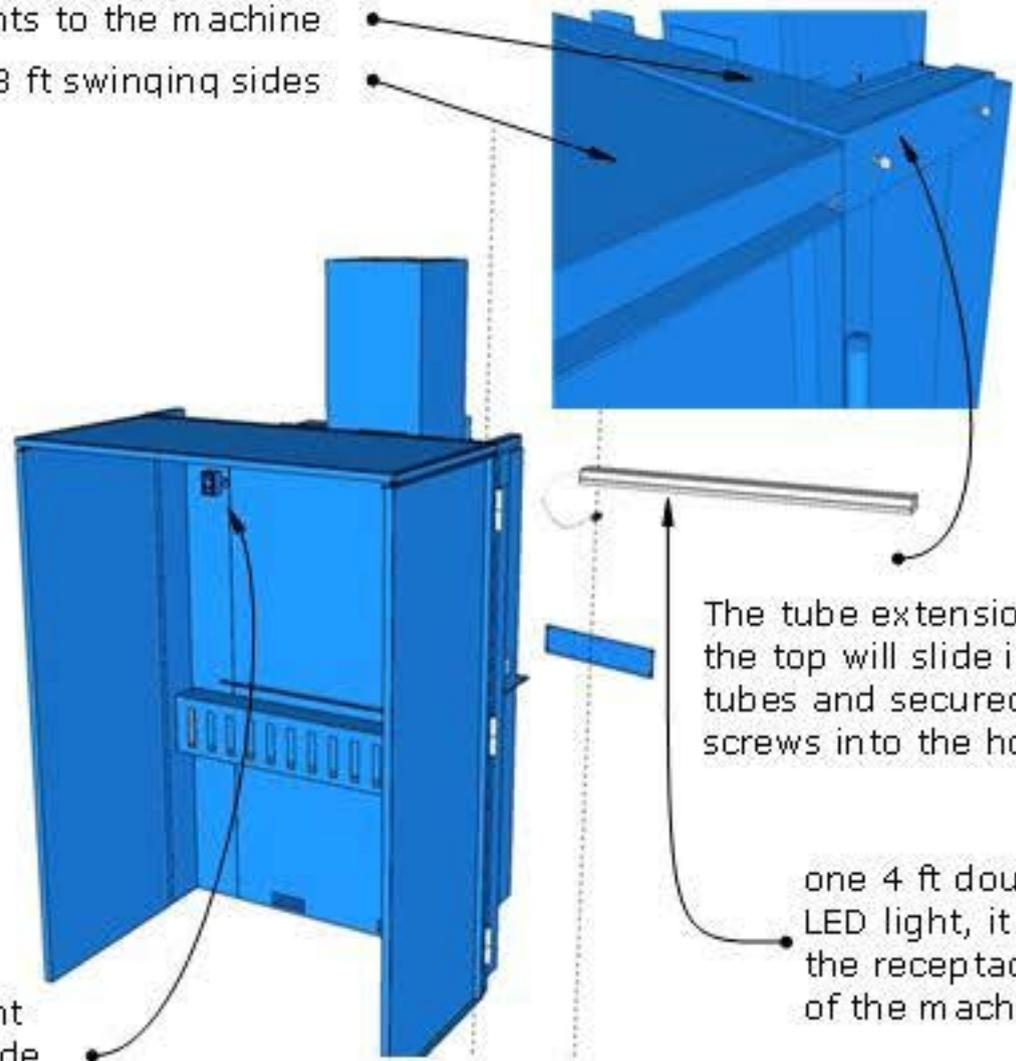
The tube extensions from the top will slide into these tubes and secured in with screws into the holes
