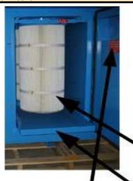
The filters will clean better with machine off, you may shut machine off and before it slows down to a complete stop, pulse the filter and allow the fan to prevent the dust from exiting the filter compartment.
