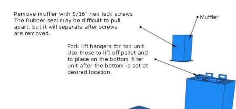
Fork lift pockets for bottom also can move the complete machine via these holes
