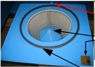
This Vee will align into the filter placed in first
